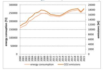
Fig. 3-26 Comparison of energy consumption and CO₂ emissions from road there was a decrease to 17 189 kt due transport to COVID situation. It was the first drop
